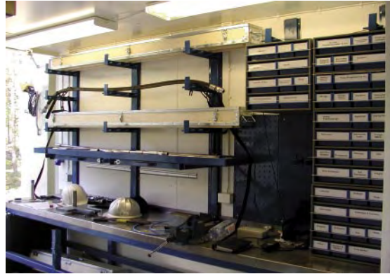
Photo 2. Rack for pump, down-hole equipment, workbench and drawers for tools.
