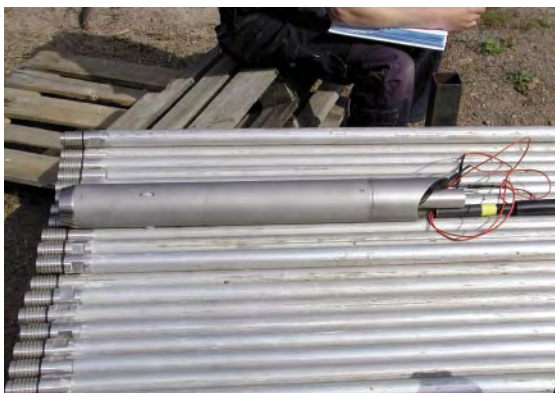
Photo 5. Positioner, bottom end of down-hole string.
