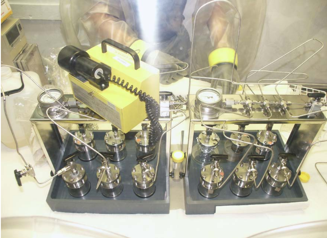
Figure 4-10 Steel oedometers with compacted bentonite were connected to KJ0052F03 in two series. All experiments were performed inside an anaerobic box at the -450 m level in the Microbe laboratory /Masurat and Pedersen 2004/.
