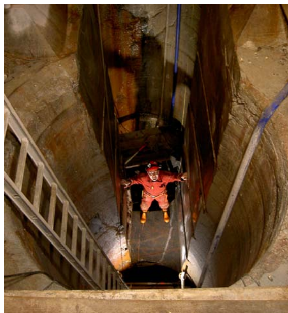
Figure 2-4 Photography of the experimental site after removal of the five one metre high pillar blocks between the two large holes.
