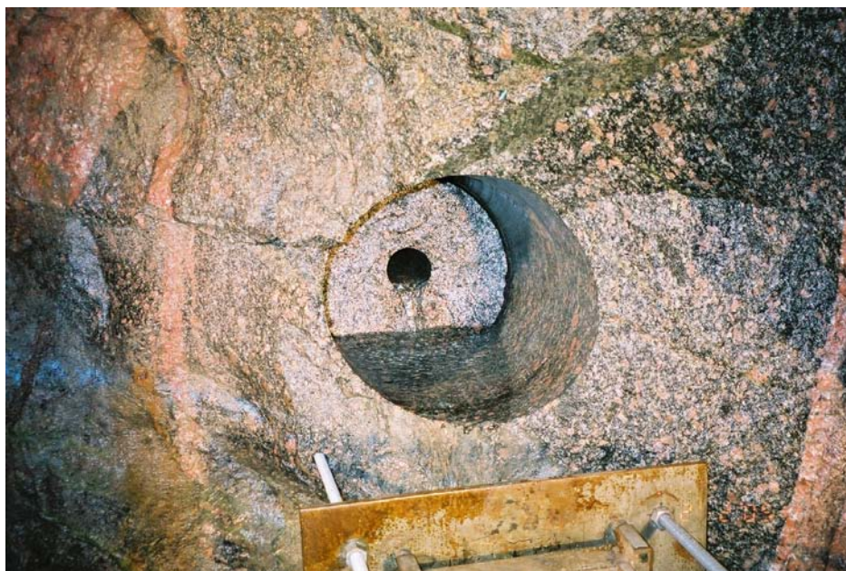
Figure 5-8 One of the five drilled boreholes in the niche.
