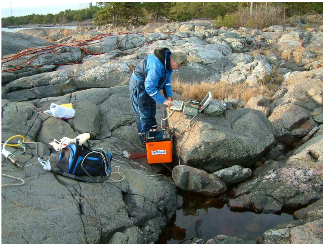
Figure 3-15. Recording instrument for seismic refraction survey conducted off the Simpevarp Peninsula and Ävrö in the late autumn of 2003 /Lindqvist 2004a/.
