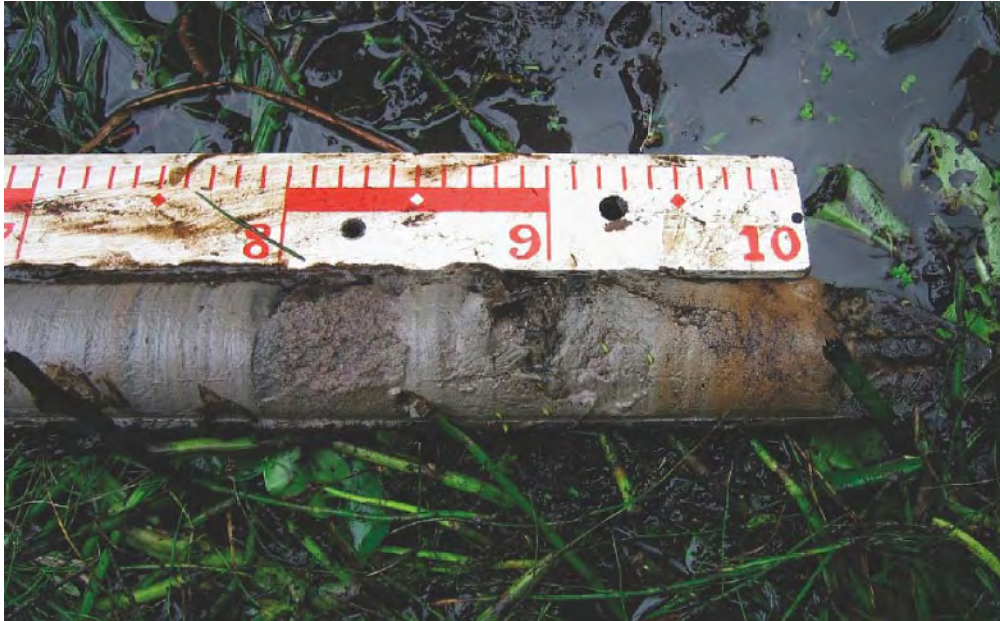
Figure 3-5. Sandy/silty layer at a depth of 280–300 cm in one of the investigated wetlands in the area /Nilsson 2004/.
