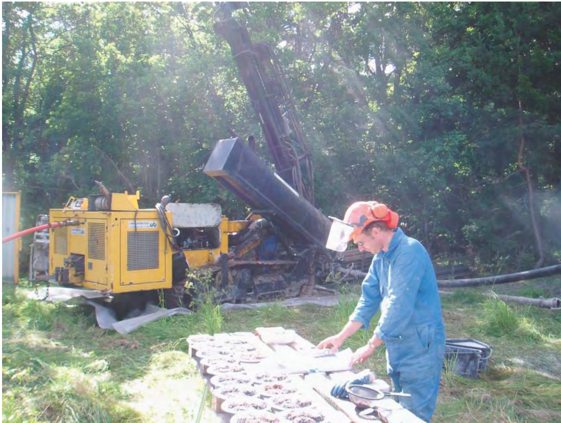
Figure 3-40. Percussion drilling and mapping of drill cuttings in HLX17.
