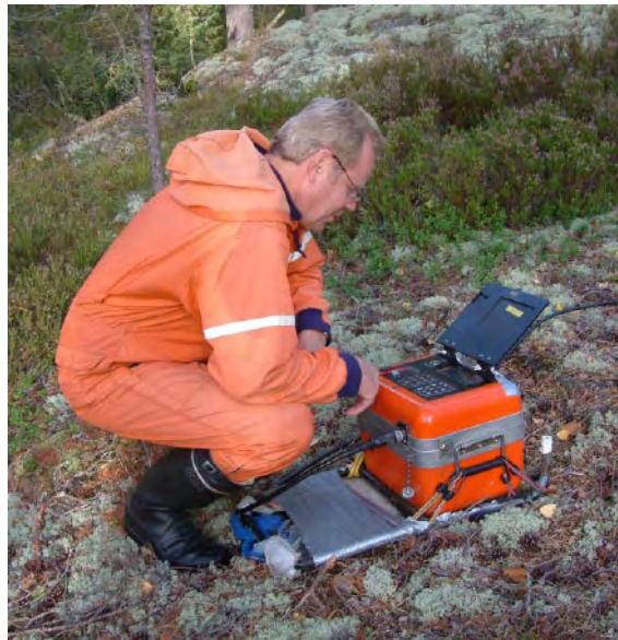
Figure 3-20. Measurement with TEM (transient electromagnetic sounding). The sketch at the left shows the principle with a transmitter (a large closed loop of cable) and a receiver (a coil). The photo at the right shows an operator at the instrument, which has been placed next to the receiver coil.
