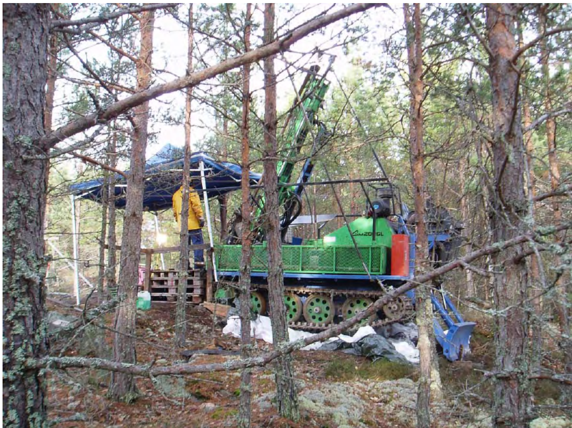
Figure B-4. Light drilling machine for drilling of short boreholes.
