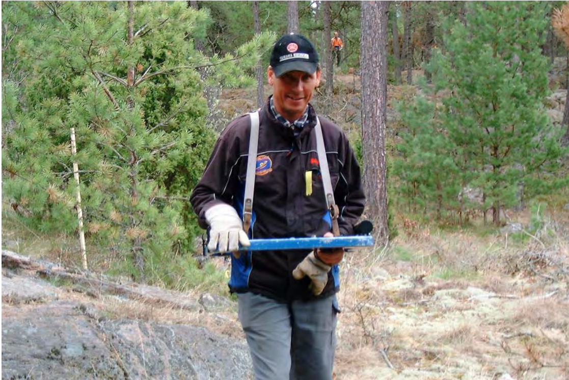
Figure 3-16. Two coils, a transmitter and a receiver, are used for electromagnetic methods such as slingram. An electromagnetic field is transmitted from the transmitter. If there is a fracture zone in the rock that conducts electric current, for example if it contains clay minerals or water, a new field is created due to electric currents generated by the transmitter field. The new field can then be detected in the receiver as a change /Triumpf 2003/.
