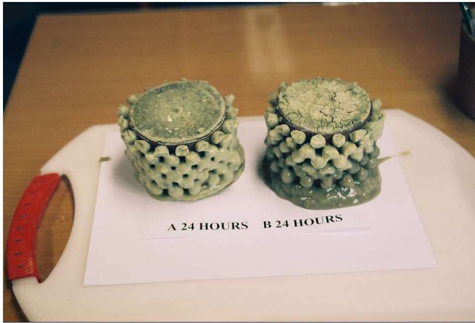
Figure 4. The plugs after 24 hours in water except for the uppermost parts. Most of the clay columns in Plug A protrude by about 6 mm and by 8-10 mm in Plug B. A very soft clay gel reaching out to about 10 mm from the tube tended to flow down along the tube in Plug B.
