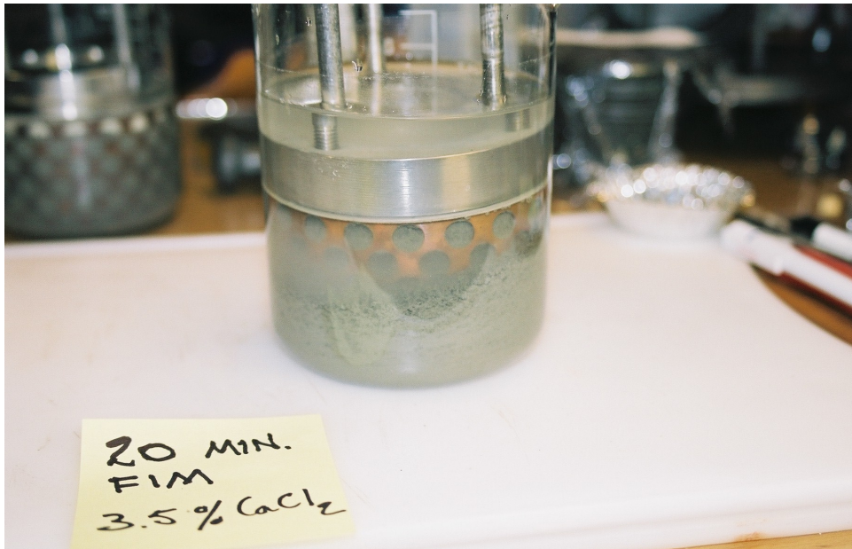
Figure 5-3. Typical quick disintegration of compacted clay plug (FIM, dry density 2280 \text{ kg/m}^3 ) submerged in salt solution (3.5 % \text{CaCl}_2 ). The clay formed around the tube in 20 minutes consists of large, soft aggregates that settle and are easily eroded.
