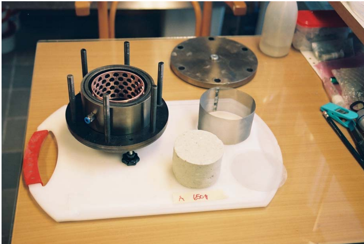
Figure 5. Oedeometer cell with perforated copper tube, steel filter and compacted clay core. Teflon coating gave the dark colour of the cell.
