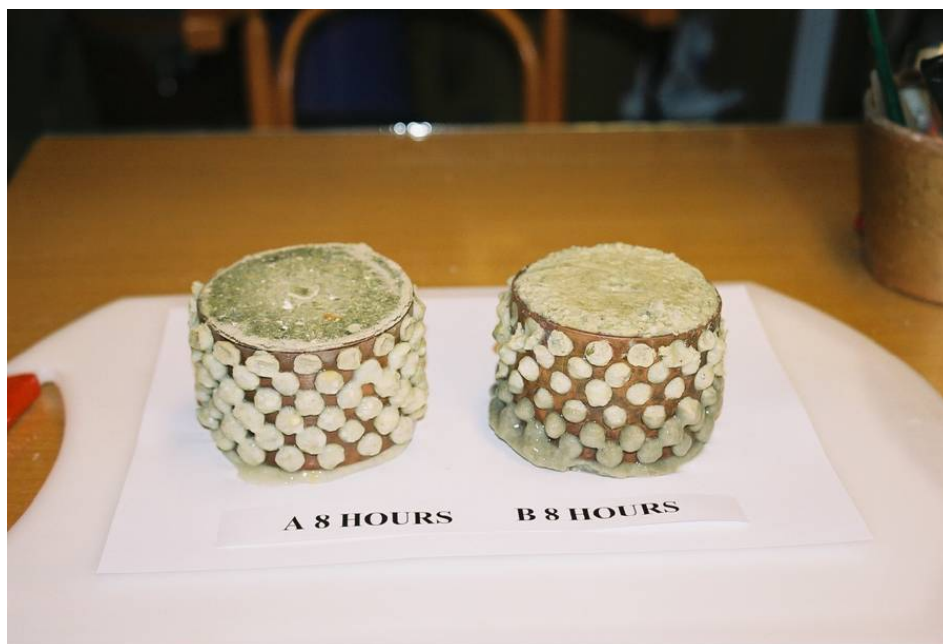
Figure 3. The plugs after 8 hours in water except for the uppermost parts. The clay columns in Plug A protrude by about 4 mm. Very soft clay gel was formed outside Plug B.
