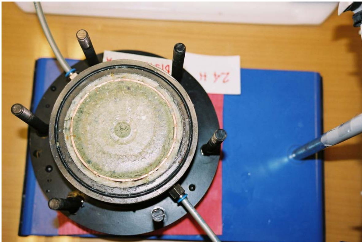
Figure 7. Appearance of the clay plug after removal of the lid 24 hours after start.
