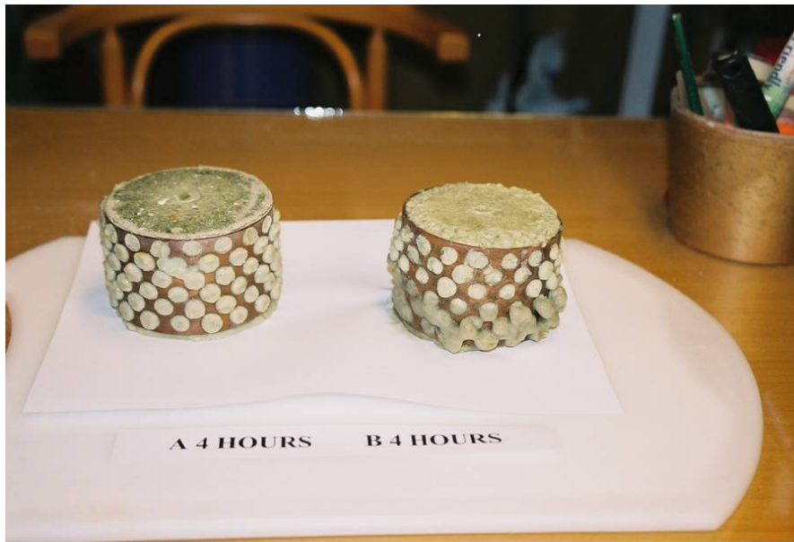
Figure 2. The plugs after 4 hours in water except for the uppermost parts. The clay columns in Plug A protrude by about 2 mm. Very soft clay gel was formed outside Plug B.
