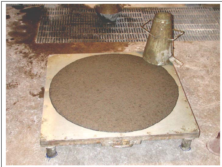
Figure 2 Picture of flow for the borehole plug concrete. This concrete is self-compacting in a borehole.
