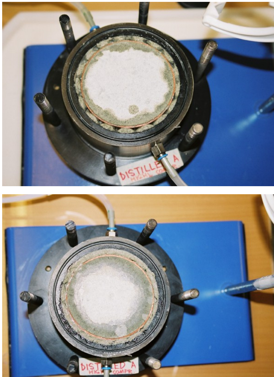
Figure 5-2. Top of perforated copper tube confining MX-80 clay with an initial dry density of 2050 \text{ kg/m}^3 in a cell with 100 mm diameter, simulating a borehole. The upper picture was taken 8 hours and the lower 24 hours after supplying the plug element with distilled water.
