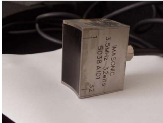
(b) The 32 element concave Imasonic array
