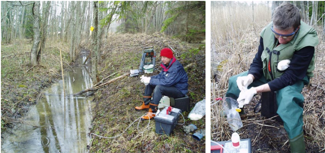
Figure 5-1. Sampling of surface water in the field. Left: In the foreground is the peristaltic pumpsystem (PPS). Right: Filtration of water in the field using a disposable filter (Millipore, 0.40 \mu\text{m} , \varnothing = 22 \text{ mm} ) and a syringe. Söder Bredviken PFM 000073 .
