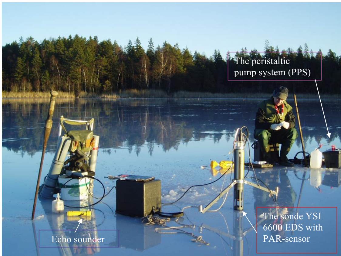
Figure 4-3. Field equipment used during sampling at Lake Eckarfjärden (PFM 117) 2004-12-07. In the foreground are the echo sounder and the YSI 6600 EDS sonde with PAR-sensor. In the background is the peristaltic pump system (PPS) used to fill sample bottles.
