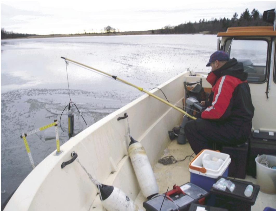
Figure 5-2. Measuring a profile (PFM000064) in the ice covered Baltic Sea with the multiple sonde (YSI 6600 EDS).
