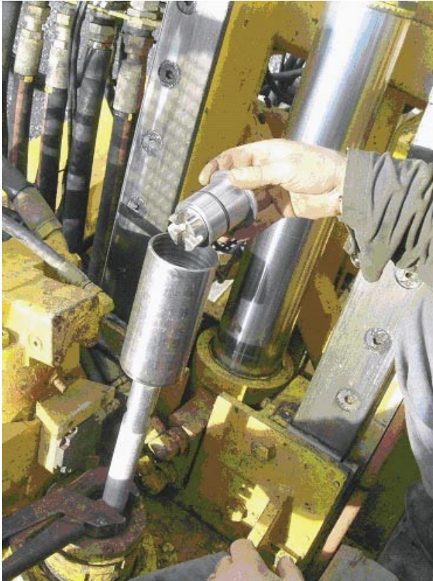
Figure 5-7. The bottom valve and its emplacement in the N-size drill stem. The 33 mm aluminium pipe can be seen below the N-sized seat for the valve.
