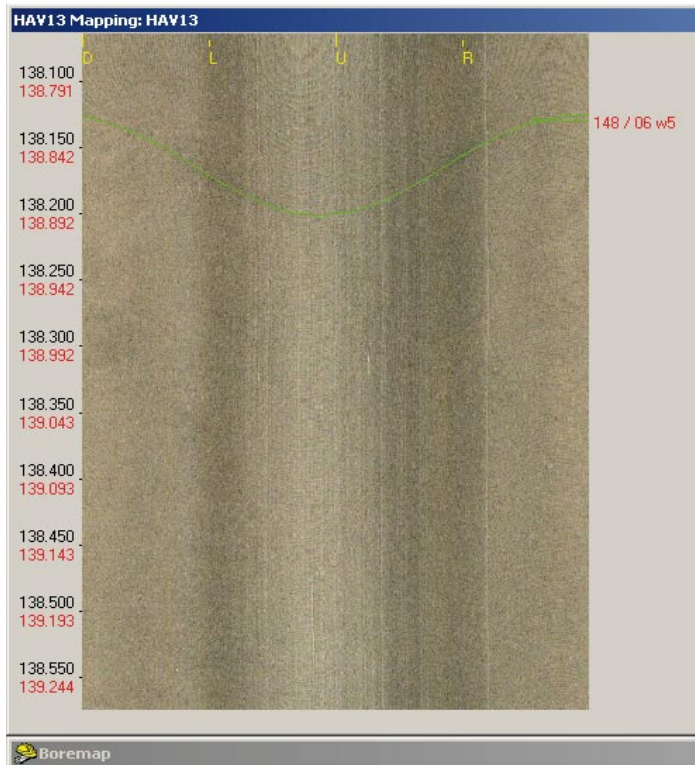
Figure 3-3. BIPS-image as it is seen in Boremap. Borehole HAV13, showing the BIPS-image at 138.8–139.3 m adjusted length, with almost no visibility because of mud in suspension and on bottom of borehole wall, one possible (uncertain) open fracture marked (green line).
