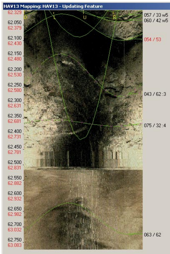
Figure 5-4. BIPS-image as it is seen in Boremap. Borehole HAV13 showing crush zone at 62.385–63,006 (adjusted length). The image of rock is very dark (very poor visibility), partly because of light colored mud on bottom of borehole wall (covers > 50% of borehole wall). There is mud in suspension at bottom of crush zone making the lower end of the zone very uncertain, so width of crush zone is uncertain.
