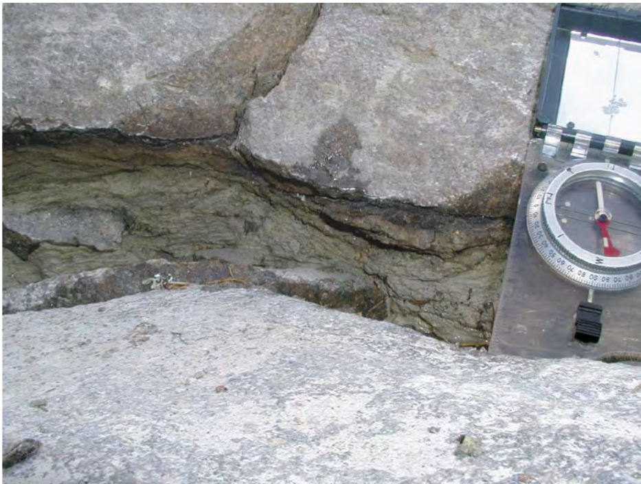
Figure G-1. Silt layer with rock fragment in horizontal fracture (photo: Kaj Ahlbom). The material is very firmly consolidated but has been slightly loosened up at the surface in this case.
