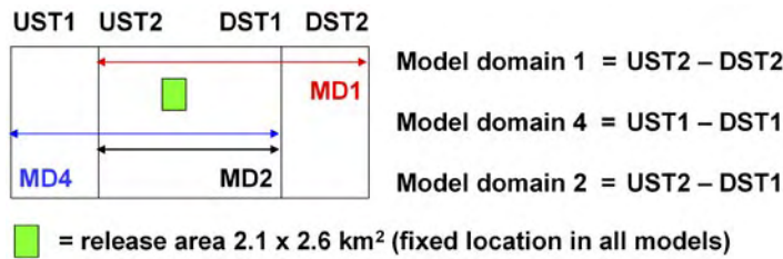
Figure 7-7. Illustration showing the approach used to test the sensitivity to the size of the model domain. UST and DST mean ‘upstream boundary’ and ‘downstream boundary’, respectively. There are two of each corresponding to the different model domains, MD1, MD2 and MD4. MD1 represents the regional model domain of version 1.2. MD2 represents a diminished model domain with a different downstream boundary than MD1. MD4 is as large as MD1 but shifted 5 km to the southwest. The green area in the centre has the same location in all model domains. Within this area 2,184 particles are released at the time slice 2,000 AD. All lateral boundaries are assumed no-flux.
