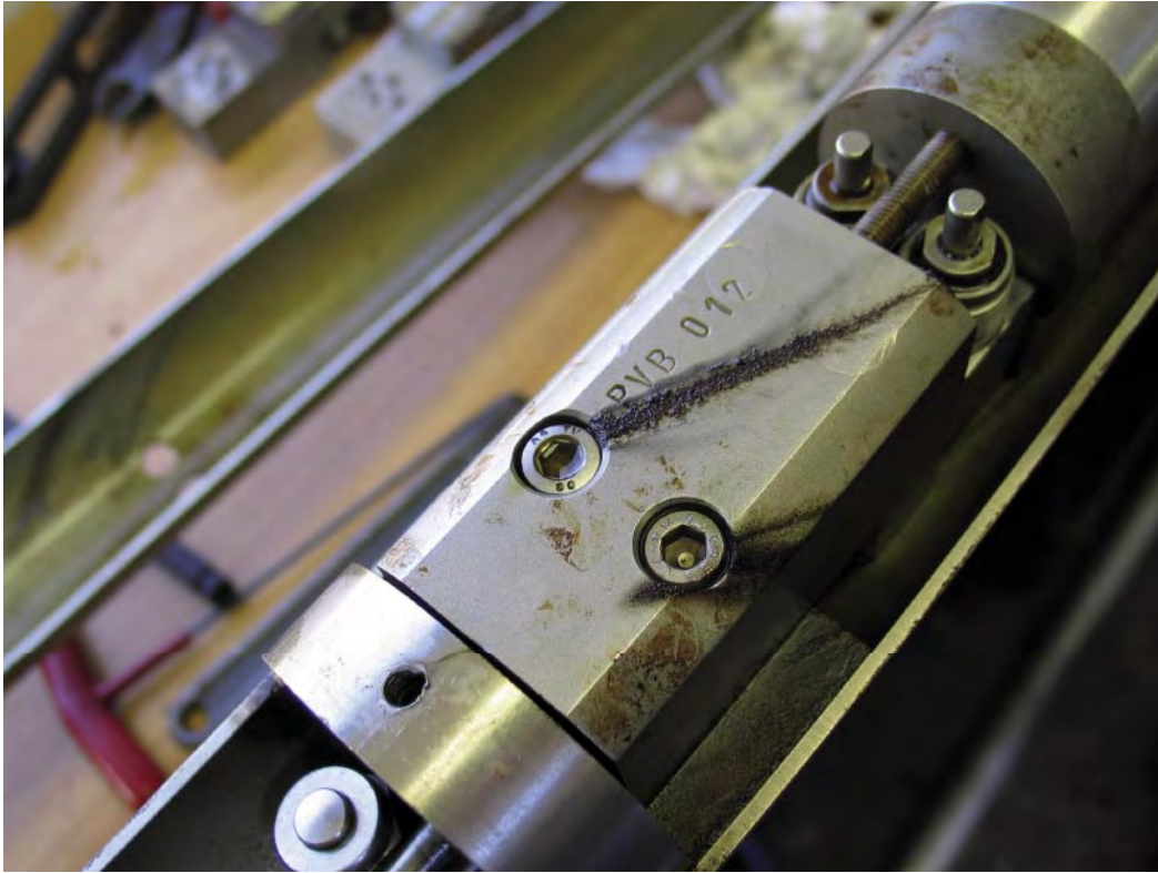
Figure 2-7. Details with crevice corrosion inside the chemical analysing equipment.
