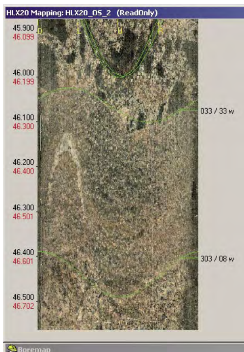
Figure 5-1. BIPS-image as seen in Boremap of borehole HLX20 between approximately 45.9–46.6 m. Weakly altered (oxidized) and somewhat porphyritic Ävrö granite containing fine-grained diorite-gabbro fragments is cut by a fine-grained granite dyke. Two open fractures are marked with green lines, as well as the borders of the dyke.
