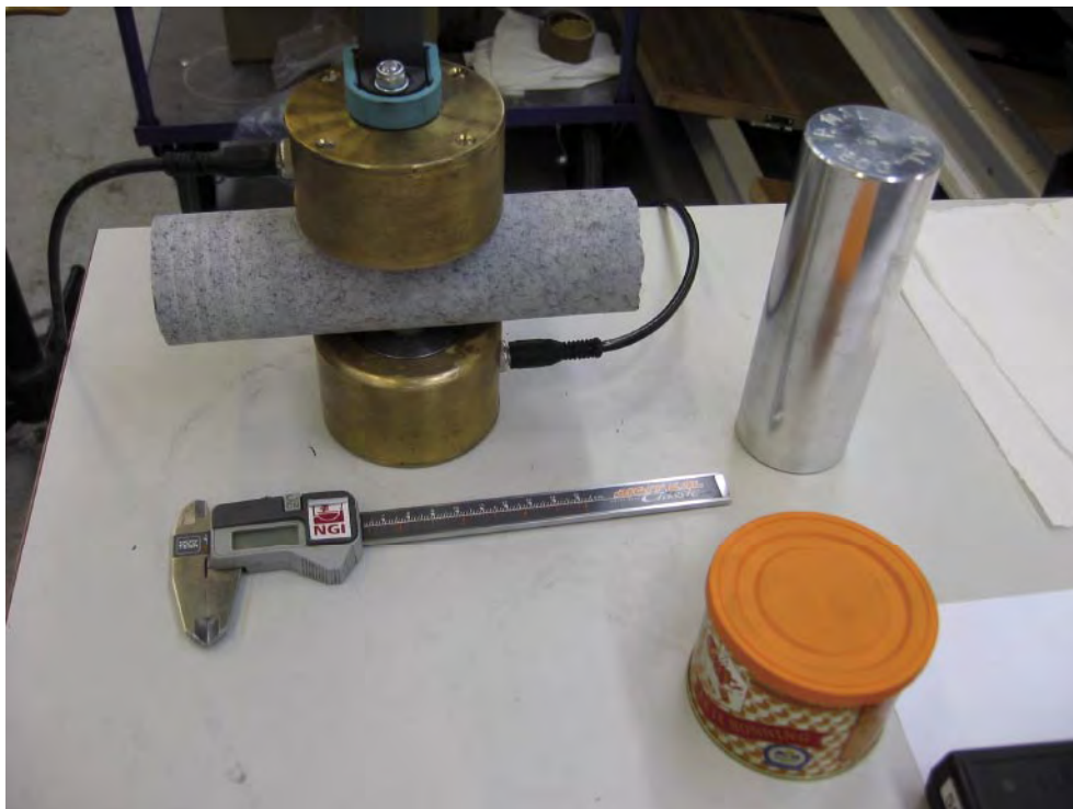
Figure 3-1. Detail of NGI's apparatus for measuring acoustic P-wave travel time transverse a foliated borehole core. The aluminium cylinder for calibration of the device is on the right.
