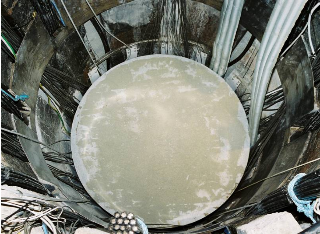
Figure 5.3-8. The deposition hole after placement of block C2.
