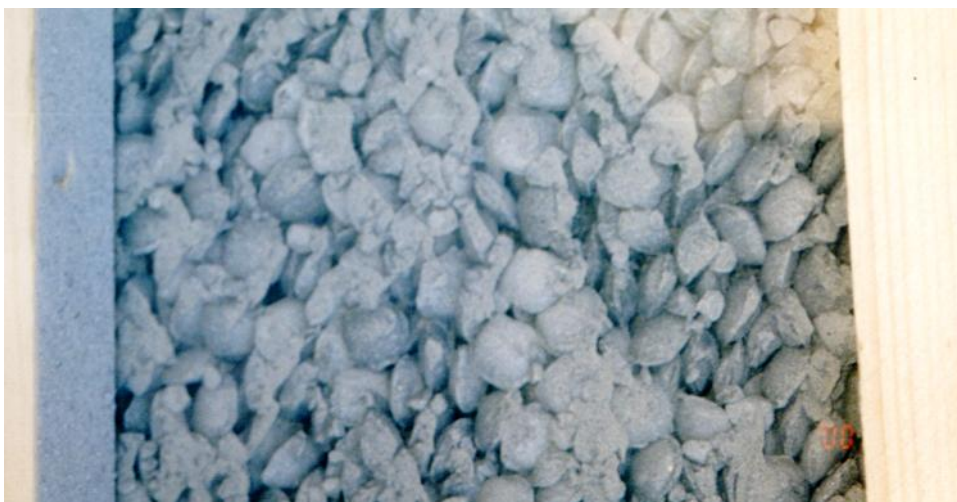
Figure 4.4-5. Bentonite pellets after filling a gap behind a Plexiglas wall.
