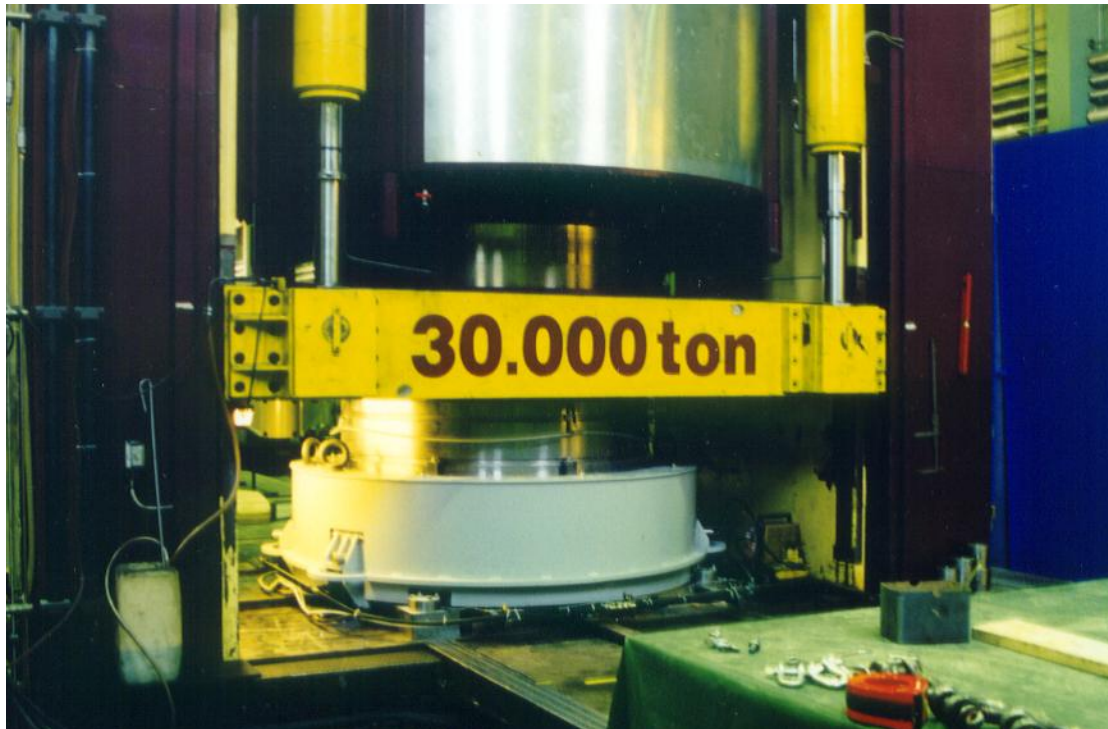
Figure 4.4-3. The compaction equipment at Hydroweld.
