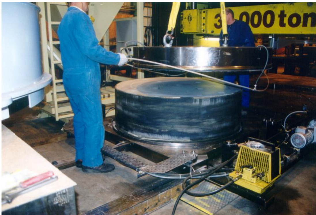
Figure 4.4-4. A bentonite block shown during removal of the mould.
