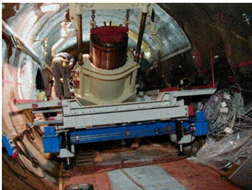
Figure 5-16. Equipment for future remote placement of SF canister in KBS-3V boreholes [5-13].
