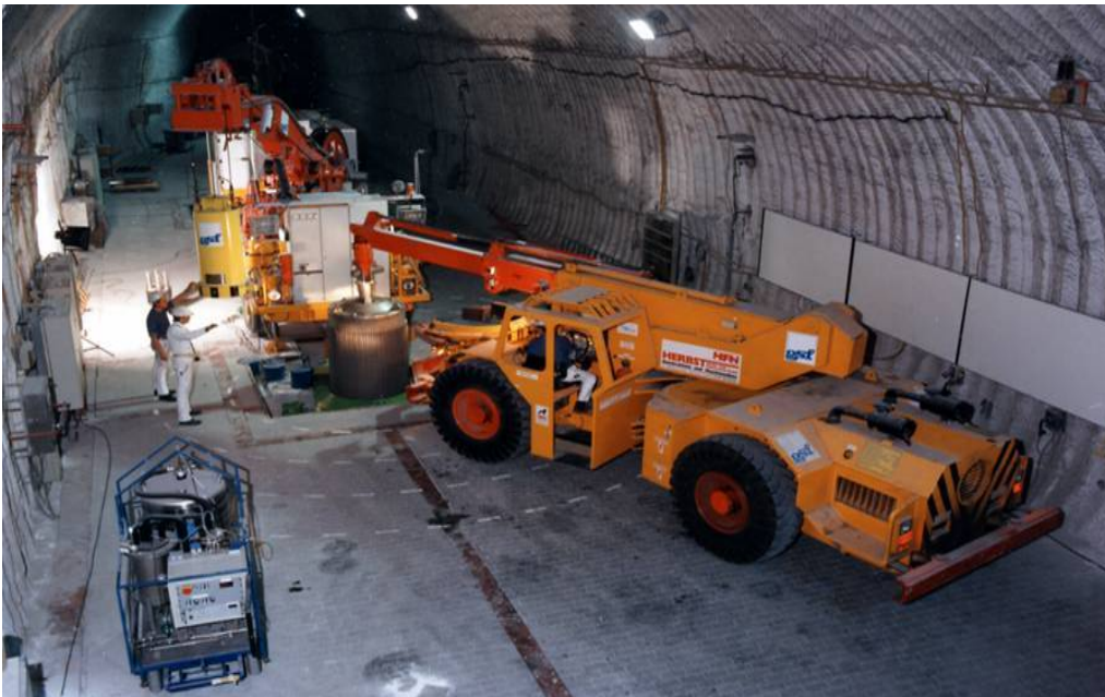
Figure 4-30. Testing of a HLW disposal system/concept in the Asse mine/URL.
