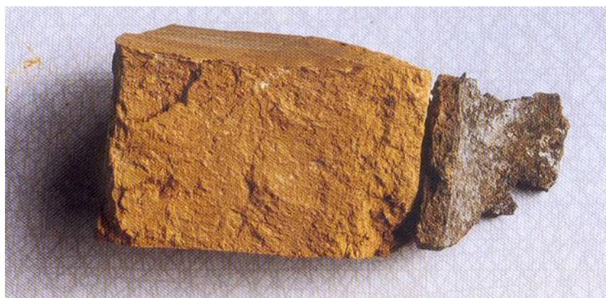
Figure 5-34. Appearance of FoCa-7 clay buffer after termination of an almost 4 year long buffer clay test in the Stripa URL. The sector-shaped clay sample was almost 75 mm in radial direction and was in contact with an iron heater with 170°C surface temperature at the right end and with rock at the other. The dark part near the heater had converted into claystone and mineral changes had significantly changed the physical properties of the entire buffer [5-30].
