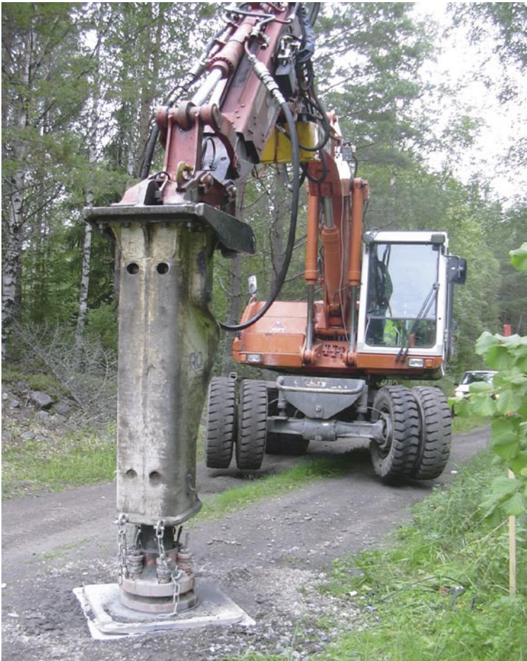
Figure 3-1. The VIBSIST-1000 seismic sources used as a seismic source at Forsmark for the 2004 VSP surveys.
