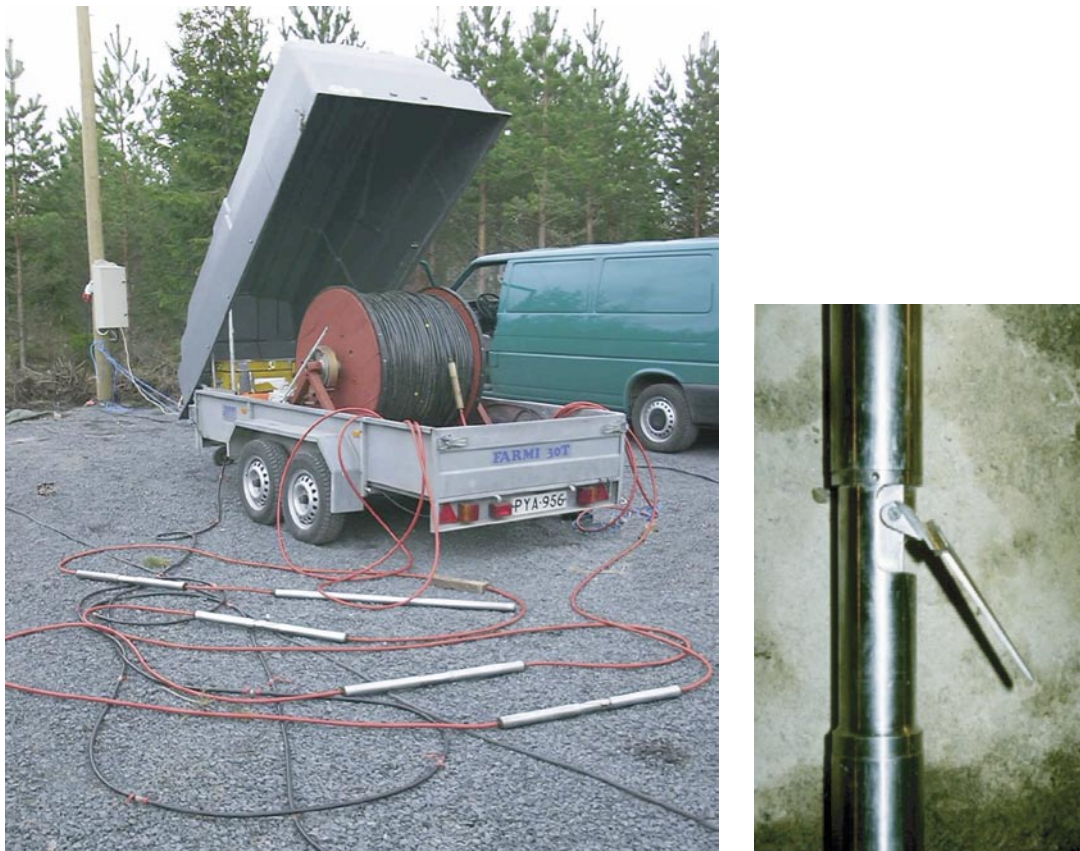
Figure 3-2. Picture of the R8-XYZ-C geophone receiver chain and detail of a 3-component module with clamping arm.
