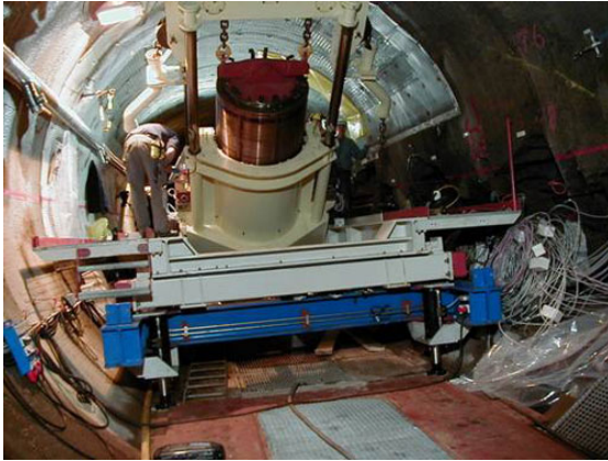
Figure 3-10. Equipment for emplacement of experimental, electrically heated canisters in KBS-3 Vertical emplacement mode. (SKB)
