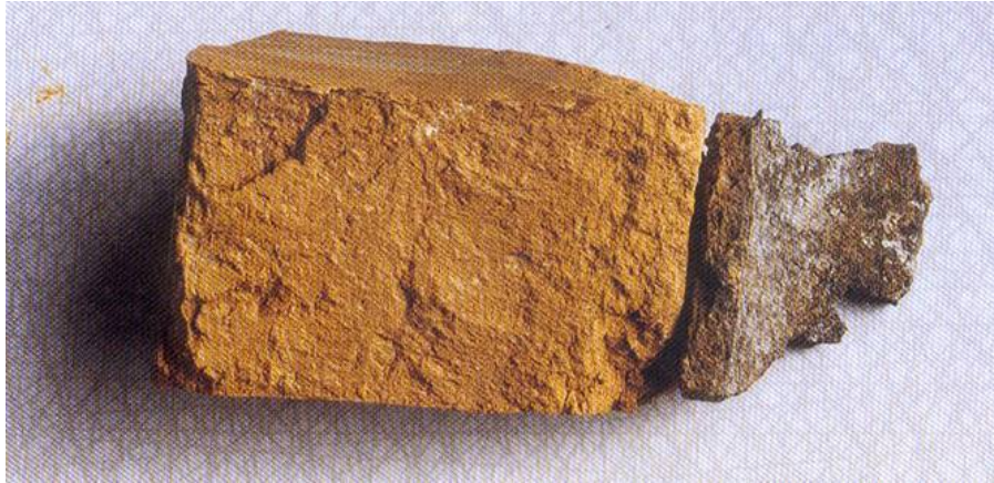
Figure 3-24. Appearance of FoCa-7 clay buffer after termination of an almost 4 year long test in the Stripa URL. The sector-shaped clay sample was almost 75 mm in radial direction and was in contact with an iron heater with 170°C surface temperature at the right end and with rock at the other. The dark part near the heater had converted into claystone and mineral changes had significantly changed the physical properties of the entire buffer. (SKB)
