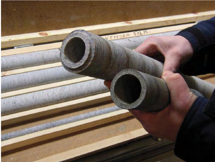
Figure 5-6. Two sections in KFM08A were tested regarding the tendency of core discing. To the left, a successfully overcored (without core discing) 62 mm core from c 519 m borehole length, and to the right, a likewise successfully overcored 51 mm core from c 543 m.
