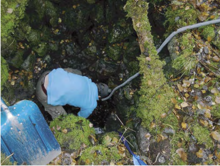
Photo no 35. Sampling point PFM002942, an old digged well, not in use for long time, had to be cleaned before any sampling action could be performed (photo A. Spets).
