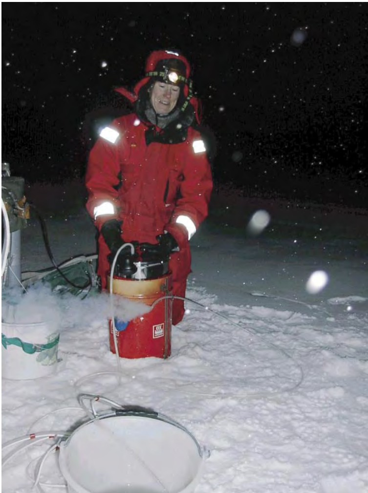
Photo no 30. Steam was a useful method to defrost the ice inside the tubes when the wheather was hard (photo J. Skarp).
