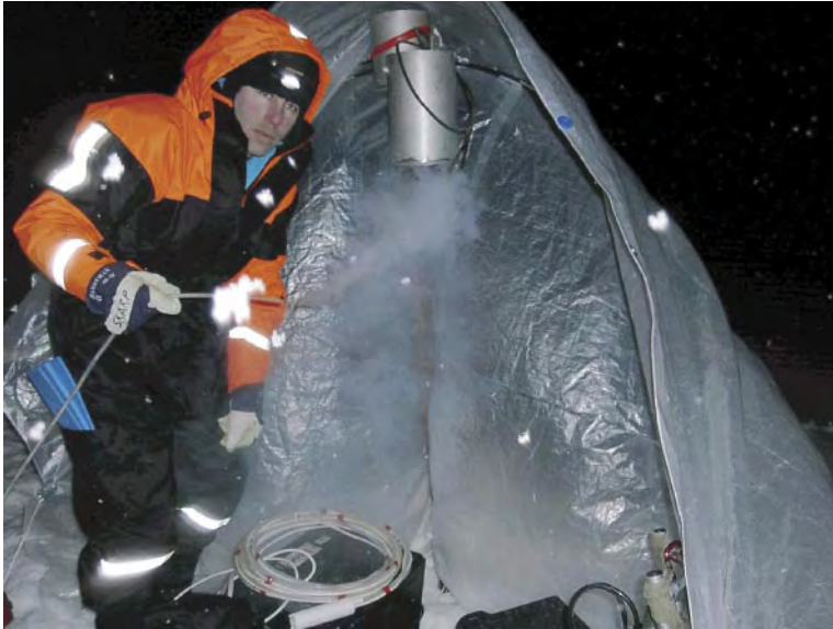
Photo no 33. Steam in action at night – trying to defrost sampling point SFM0025, Vargudden, in hard weather conditions (photo A. Spets).
