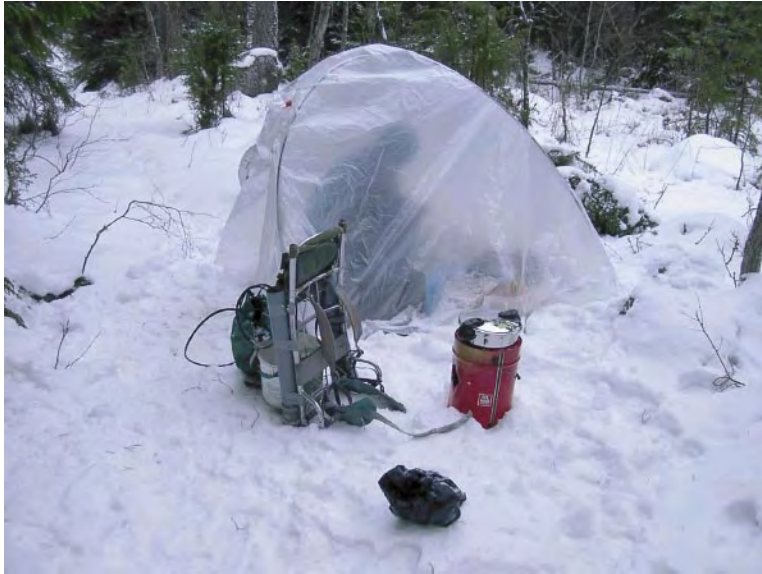
Photo no 31. A tent over the sampling object made sampling much easier in cold wheather conditions (photo J. Skarp).
