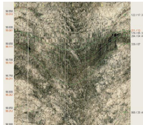
Figure 3-9 b. Crushed section at 98.63–99.10 m, mapping B.
