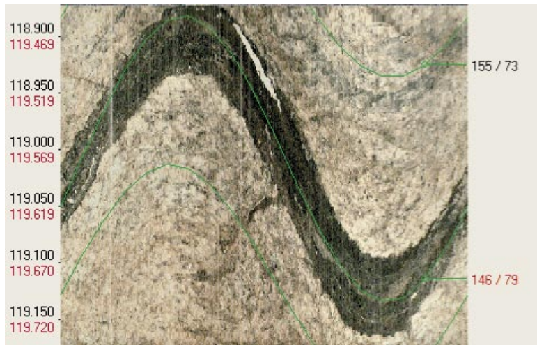
Figure 3-4. Possible mylonite at 119.01 m, mapping B.
