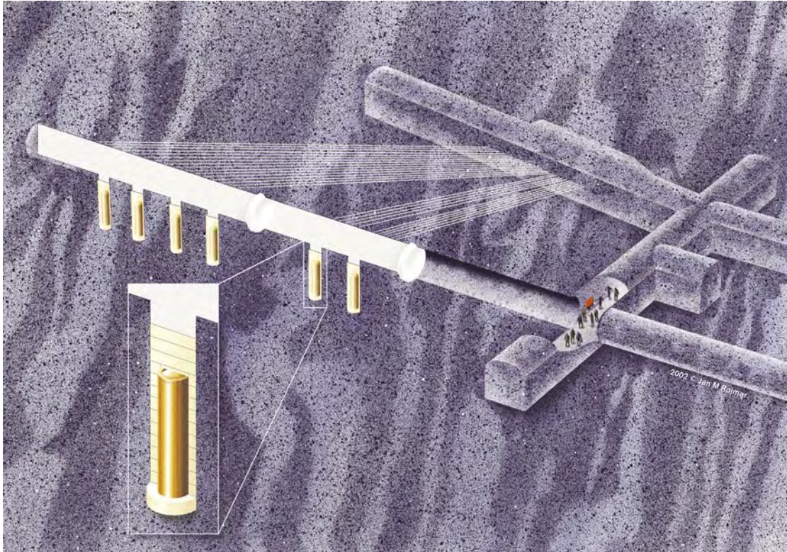
Figure 2-5. Schematic view of the layout of the Prototype Repository (not to scale).
