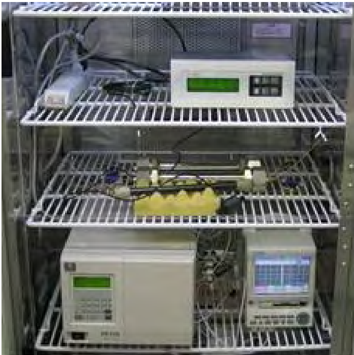
Figure 6-46. Groundwater circulation system in experimental laboratory.
