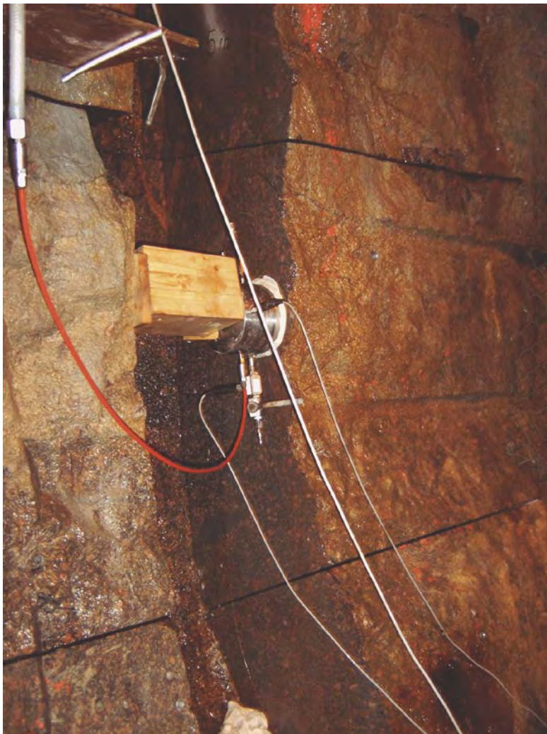
Figure 6-13. Test location of the surface packer in a slot (Q-Tunnel).
