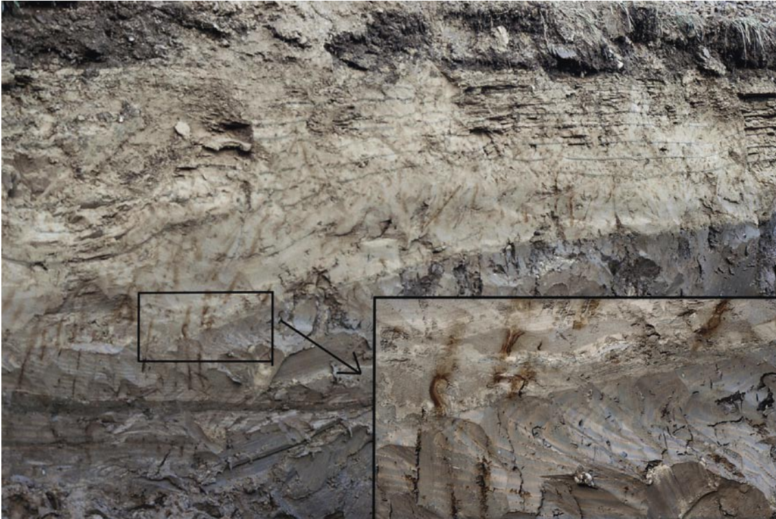
Figure 5-16. Illusory stratigraphy due to graceful sliding at Örnäs (E7 in Figure 4-1). An almost undeformed slab of thick-varved, sandy silt (light coloured with thin, dark layers of clay) has come to rest on varved glacial clay. The uppermost bed consists of cultivated topsoil rich in pebbles and cobbles. The close-up photo (lower right-hand corner) shows the slip surface with drag folds in the upper parts of the clay.
