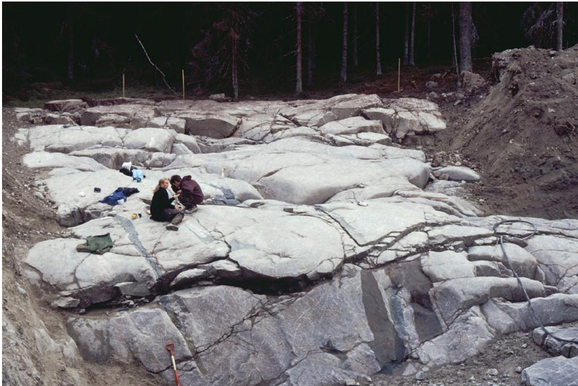
Figure 5-1. Glacially smoothed and striated bedrock exposure at deep drilling site BP5 in the candidate area at Forsmark. Fresh looking fractures occur almost all over the exposure. The major fracture (foreground), lacking signs of being affected by glacial abrasion, was filled with laminated silty and fine sandy sediments.
