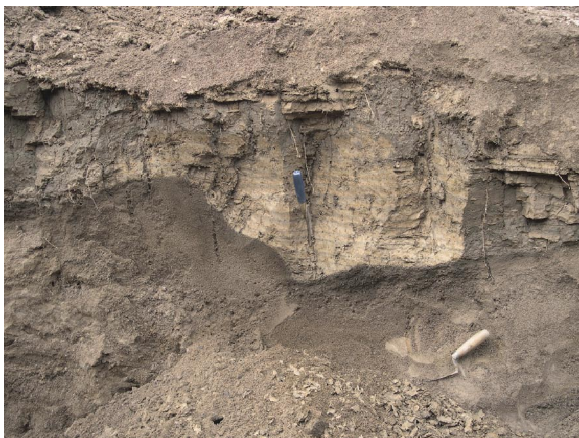
Figure 5-19. Slide deposits of non-folded glacial clay in uneven contact with underlying sandy sediments at Salsta (E13 in Figure 4-3). The dark-coloured layer along the slide surface beneath the clay is a mixture of sand and clay.
