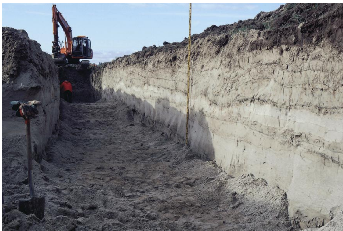
Figure 5-15. Typical of the stratigraphy along the Börstil esker, this trench section at Östansjö (E8 in Figure 4-1) shows a bed of loosely packed fine sand and coarse silt covered by a bed of clay-laminated silt. The uppermost 0.4 m consists of cultivated topsoil. Extended excavation revealed loosely packed and saturated glaciofluvial sand to a depth of at least 5 m. Although the stratigraphy is considered to be highly susceptible to liquefaction, no deformations related to seismically induced liquefaction were found here or elsewhere along the Börstil esker.
