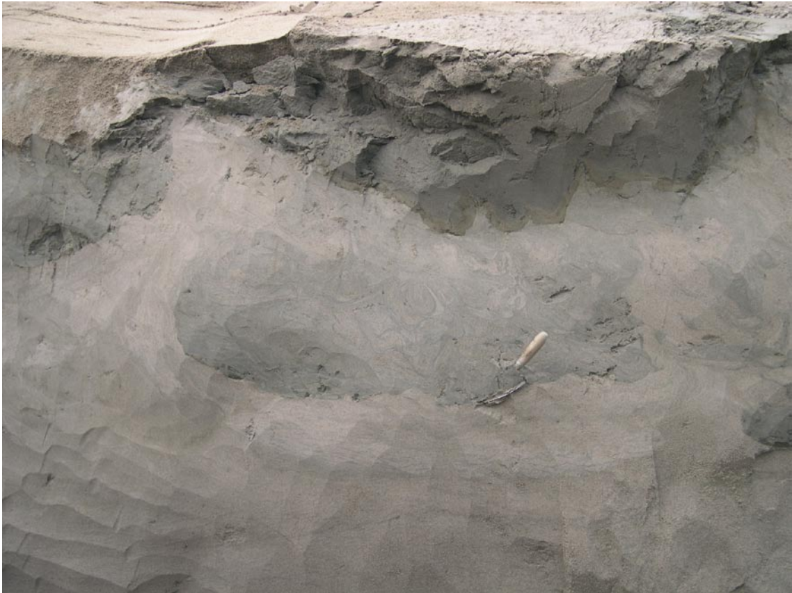
Figure 5-26. Convolute bedding, with ball-and-pillow structures and pseudo-nodules, in densely packed fine-sandy and silty sediments of glacial origin at Runhällen (E17 in Figure 4-3). The deformations are interpreted as possible effects of earthquake-induced liquefaction and dewatering.
