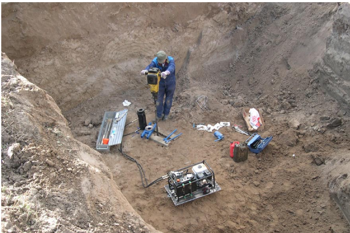
Figure 4-7. Coring provided complementary information about thickness and character of sediments at depths at Torkelsbo (E15 in Figure 4-3).
