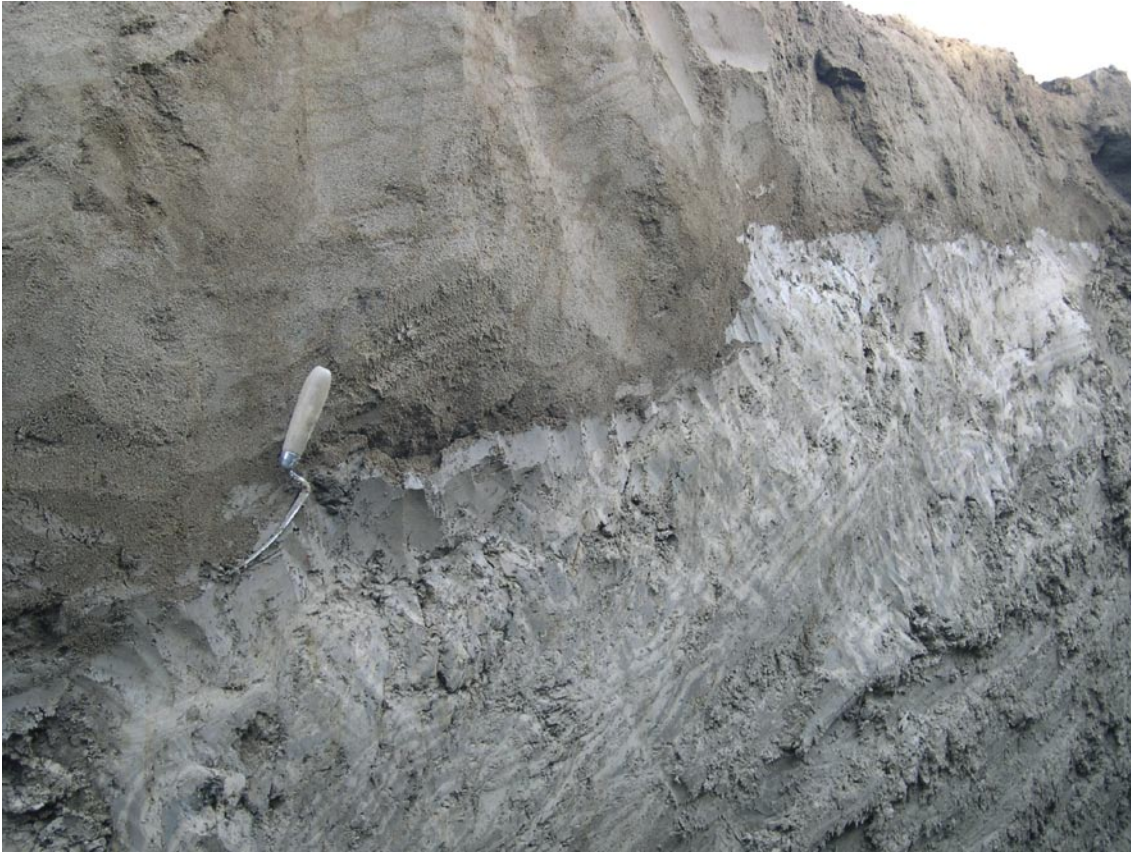
Figure 5-25. The southern part of the funnel-shaped sand filling at Torkelsbo. The folded fine-grained glacial sediments show an eroded, jagged contact against the densely packed sand.
