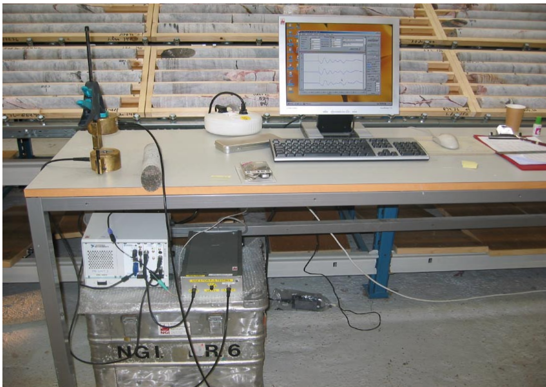
Figure 3-2. NGI's equipment set-up for measuring acoustic P-wave travel time transverse borehole core.
