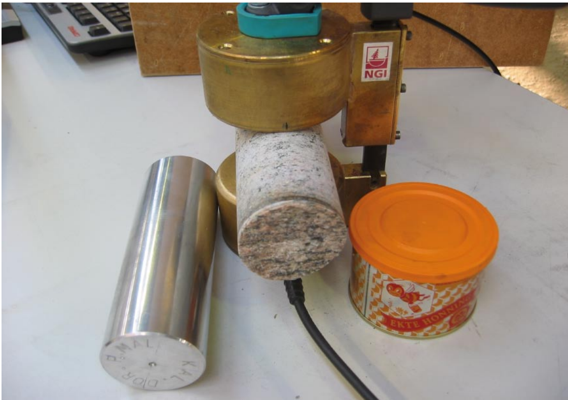
Figure 3-1. Detail of NGI's apparatus for measuring acoustic P-wave travel time transverse a foliated borehole core. The aluminium cylinder for calibration of the device is on the left.
