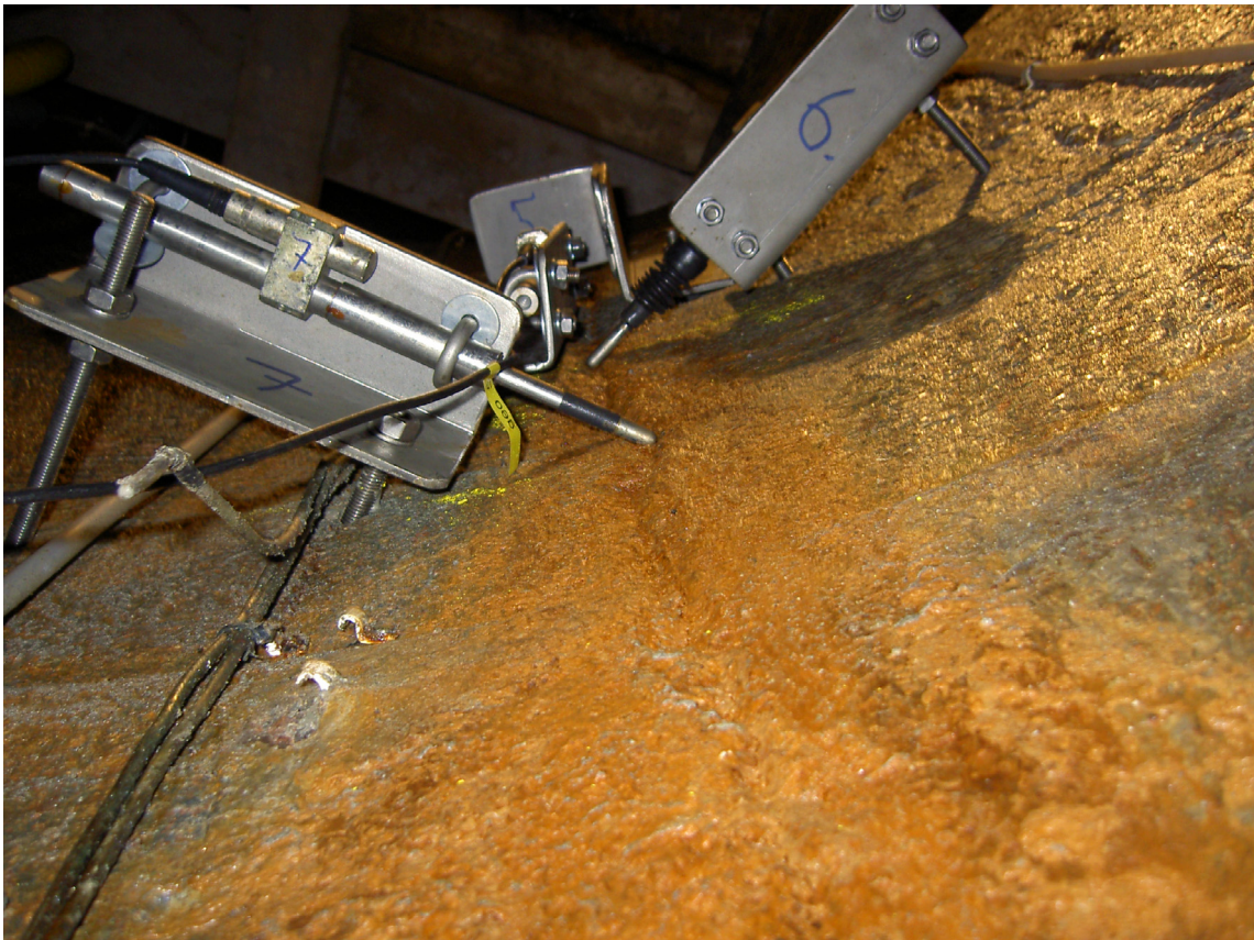
Figure 2-1. LVDTs installed on the monitored fractures view from above).
