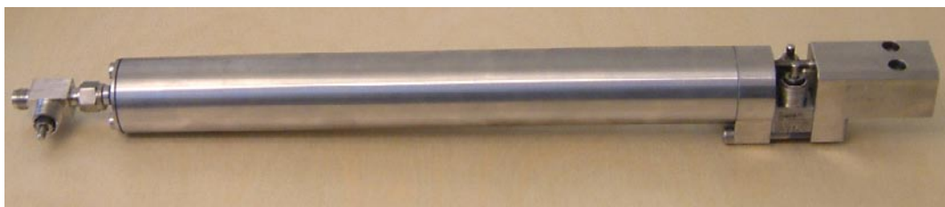
Fig. 3: SKB stainless steel sampling cylinder (left: piston side, right: mounting adapter side)
