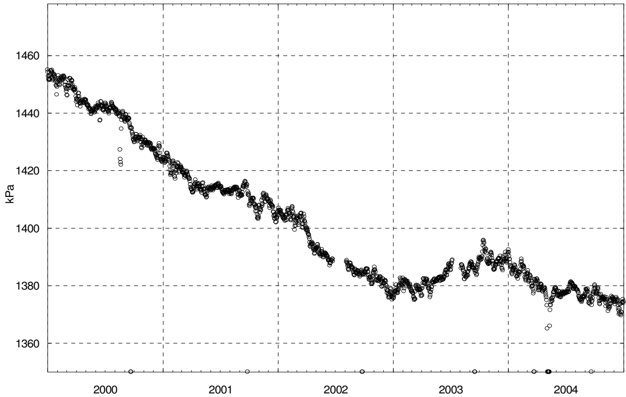
Figure 6-6 Groundwater pressure in tunnel borehole KA1061A, 2000-2004.
