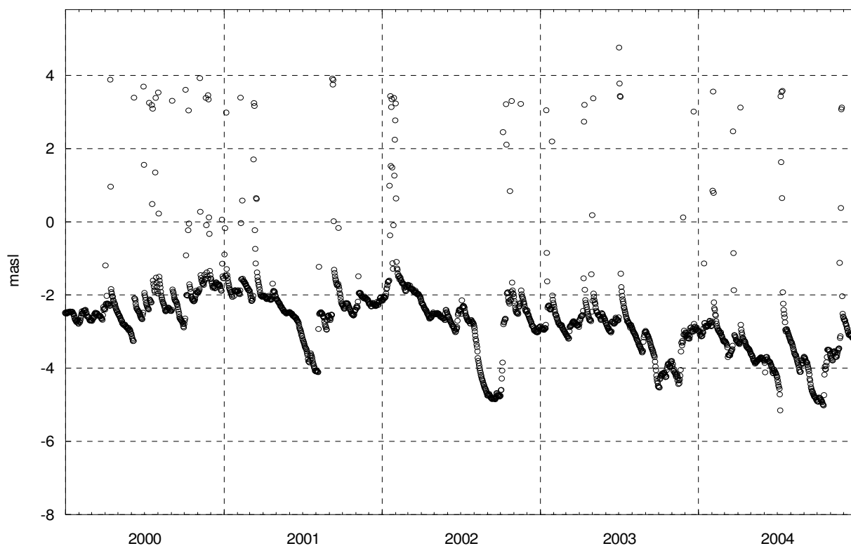
Figure 6-5 Groundwater levels in HAV08 on Ävrö, 2000-2004.
