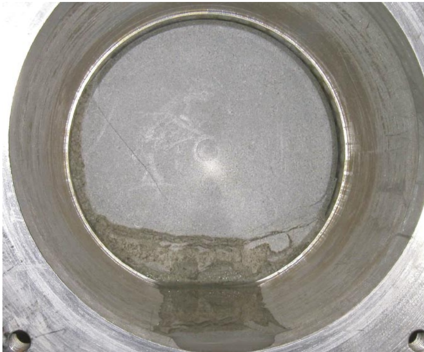
Test II-2. Picture taken outside the plug after removing the displacement sensors and the steel ring. The inflow was about 60 times lower than in Test II-1, but still the leakage and bentonite erosion was very strong.
