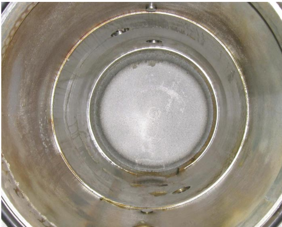
Test II-4. Picture taken from inside after removal of the PVC dummy. The end of the bentonite block is shown. The “active area” that was wetted is very clearly seen.
