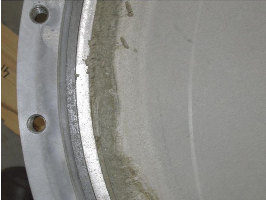
Figure BB1-9. Picture showing the radial slot filled with clay. BB1.
