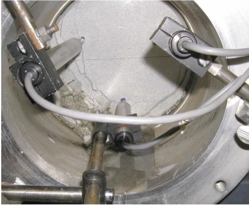
Test II-1. Picture taken outside the plug during the test. The leakage of water and the bentonite erosion is very strong.
