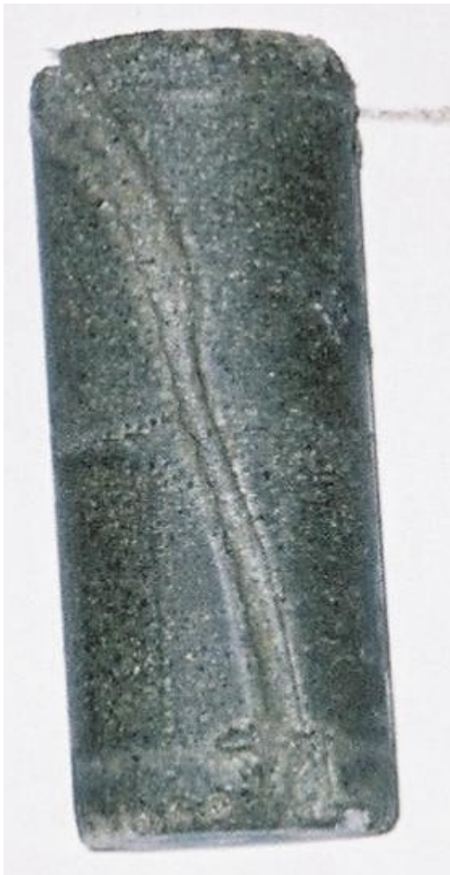
Figure 6-2. Picture of a sample where the piping did not seal.
