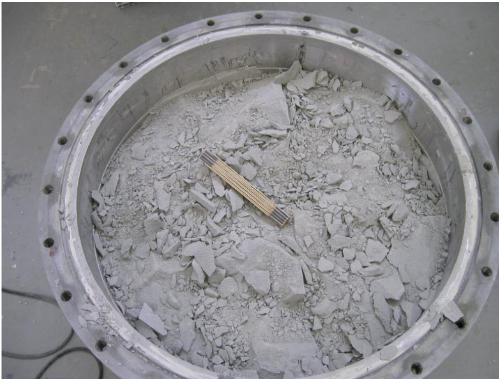
Figure BB7-5. Picture from the dismantling and excavation. Half the block is removed. Everything is dry.
