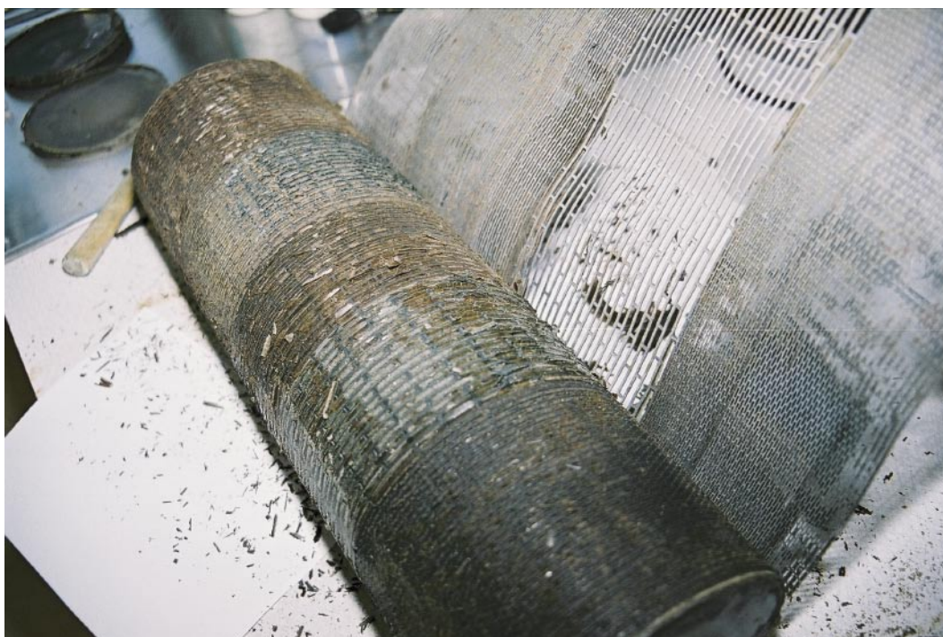
Figure 4-14. Picture of the buffer after “unrolling” the perforated steel container.
