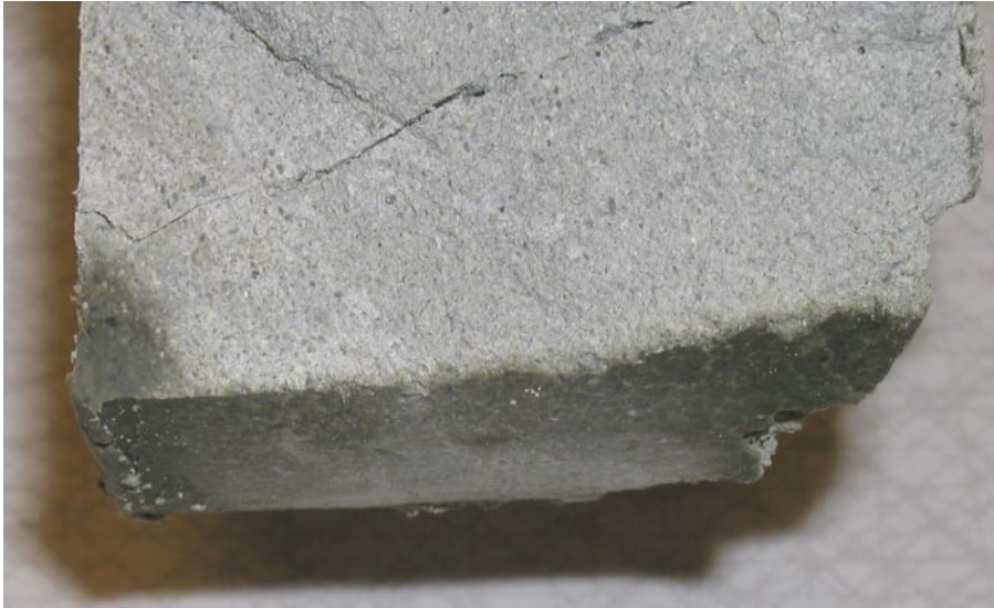
Test II-3. Picture showing a part of the distance block after dismantling of test 3. The left side faced the PVC dummy. The picture shows that only a small part of the block was active in the sealing process.
