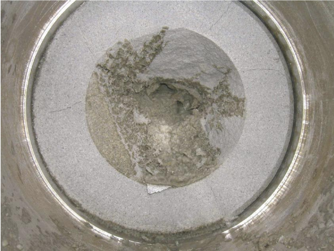
Figure 7-13. Picture from test II-7 showing the outside of the block after removal of the load cells and the steel ring. When the inner water pressure reached 2.5 MPa a central part of the distance block cracked.
