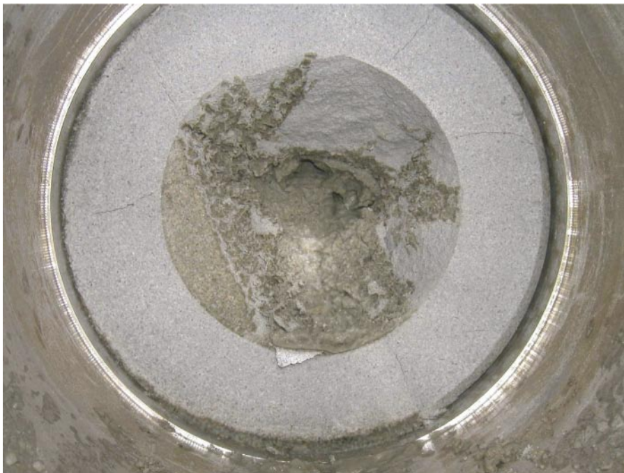
Test II-7. Picture from test II-7 showing the outside of the block after removal of the load cells and the steel ring. When the inner water pressure reached 2.5 MPa a central part of the distance block cracked.
