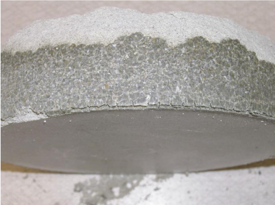
Test II-8. Picture of the wetted peripheral surface of the distance block.
