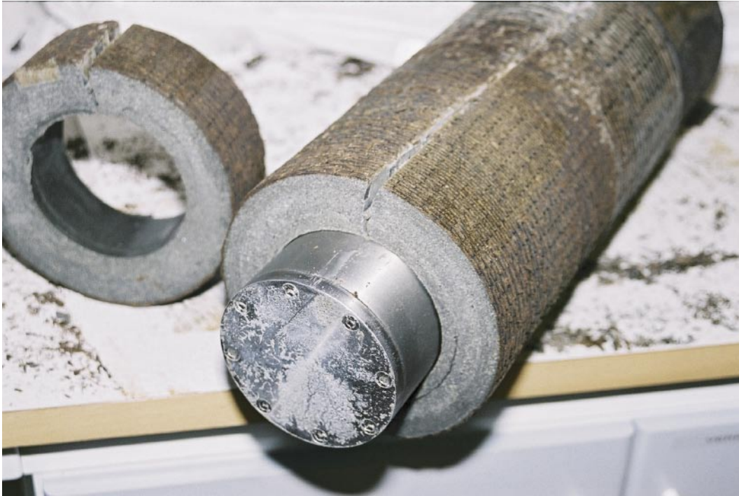
Figure 4-15. Picture taken during removal of the buffer.
