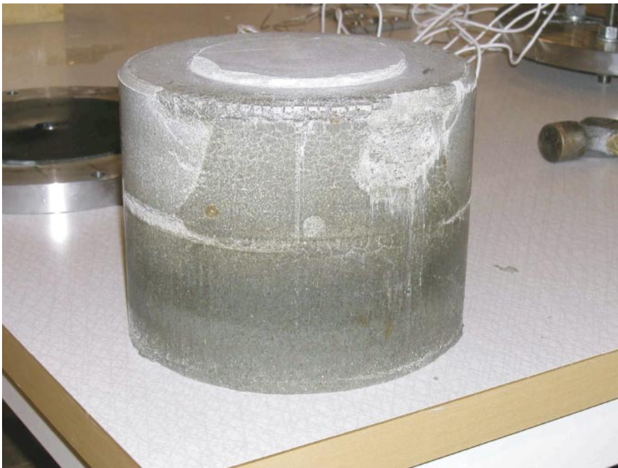
Test II-9. Picture of the bentonite blocks after dismantling. The inner block (lower in the picture) is wet all around the periphery, but the outer block is only wet on the bottom part.
