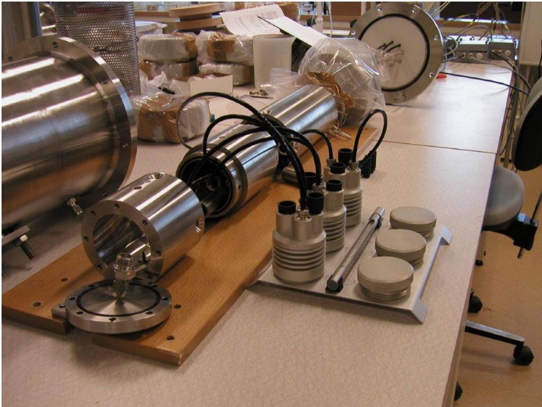
Figure 4-5. Picture showing the instrumented canister during calibration of the RH-sensors. The black cables going from the canister to the small vessels are the RH sensors, which are calibrated in the vessels before test start.
