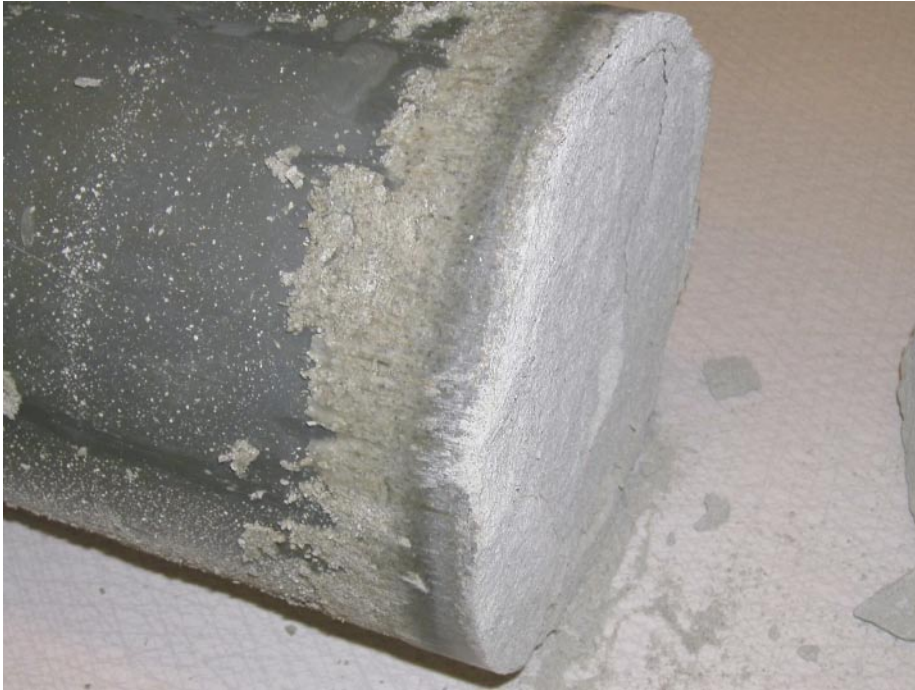
Test II-6. Picture of half the distance block and the PVC dummy taken after dismantling. When the PVC dummy was removed from the test cylinder the block was split in two parts. The sealing and the swelling into the slot along the PVC dummy is clearly seen.
