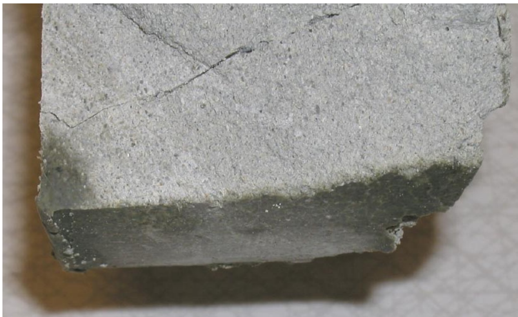
Figure 7-12. Picture showing a part of the distance block after dismantling of test 3. The left side faced the PVC dummy. The picture shows that only a small part of the block was active in the sealing process.
