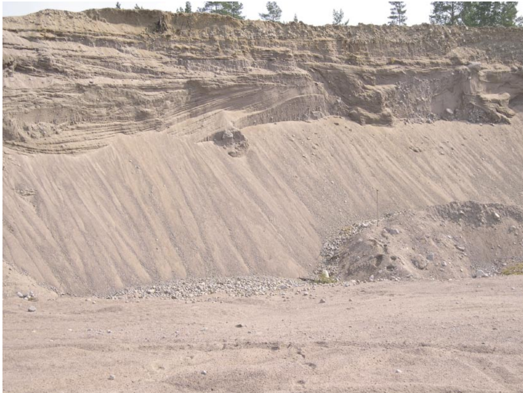
Figure 5-13. A 7 m high section in glaciofluvial sediments dominated by gravel and sand just south of lake Jämsen (PSM005621). Some internal structures as loadcast and ripples can be observed in the section.
