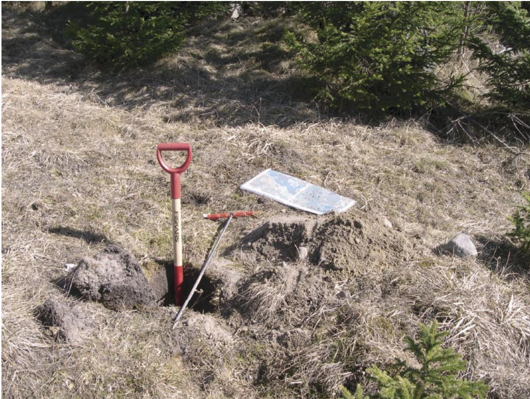
Figure 3-1. A spade and a hand-driven probe used in the field.
