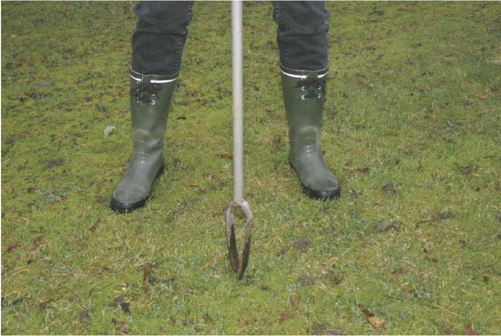
Figure 3-2. The Edelmann hand-driven probe was valuable in the field-work.
