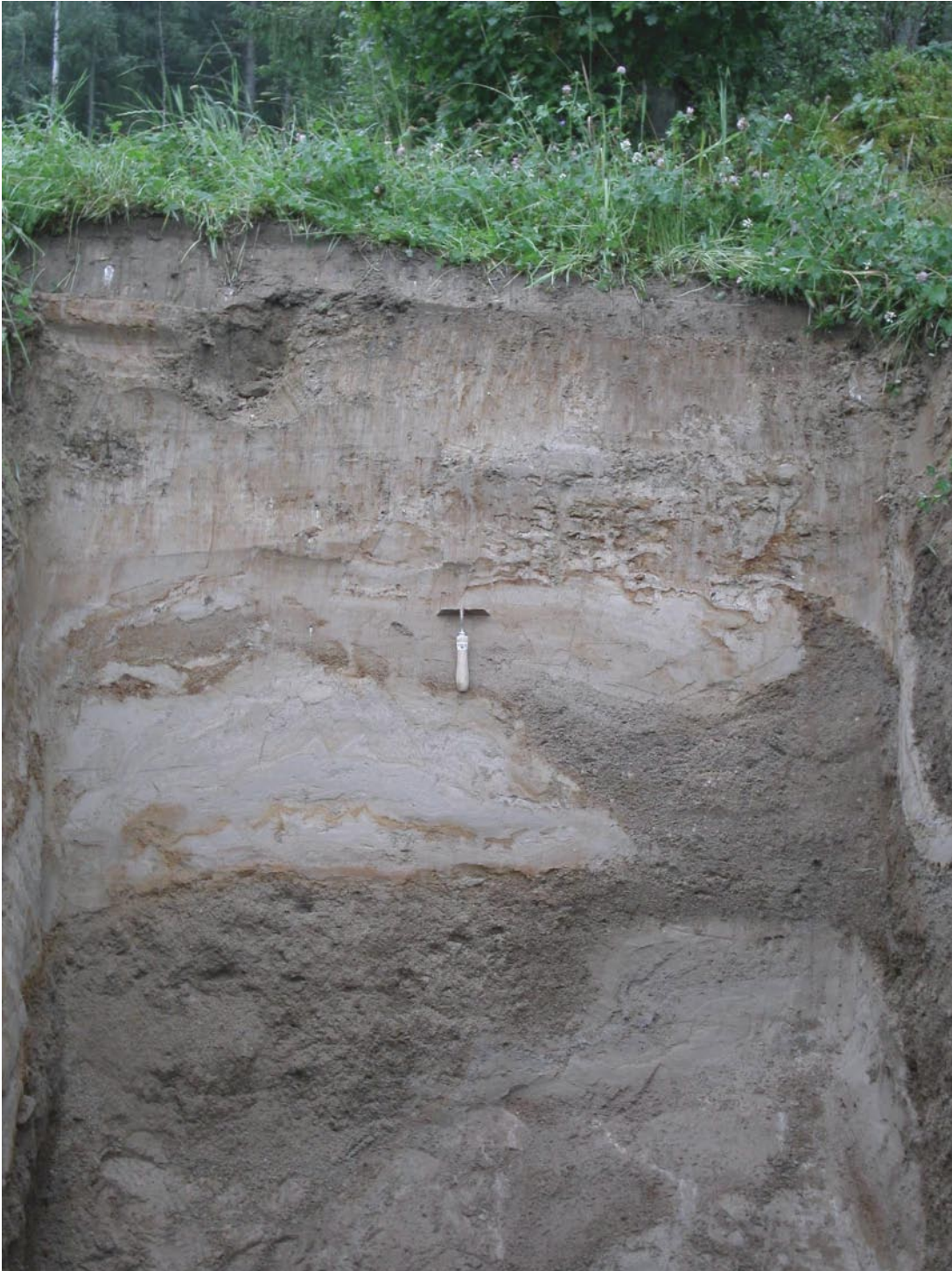
Figure 5-14. Deformed beds of glaciofluvial sand and silty sand in a section near Frisksjön (6367978 N, 1548719 E; PSM005401).
