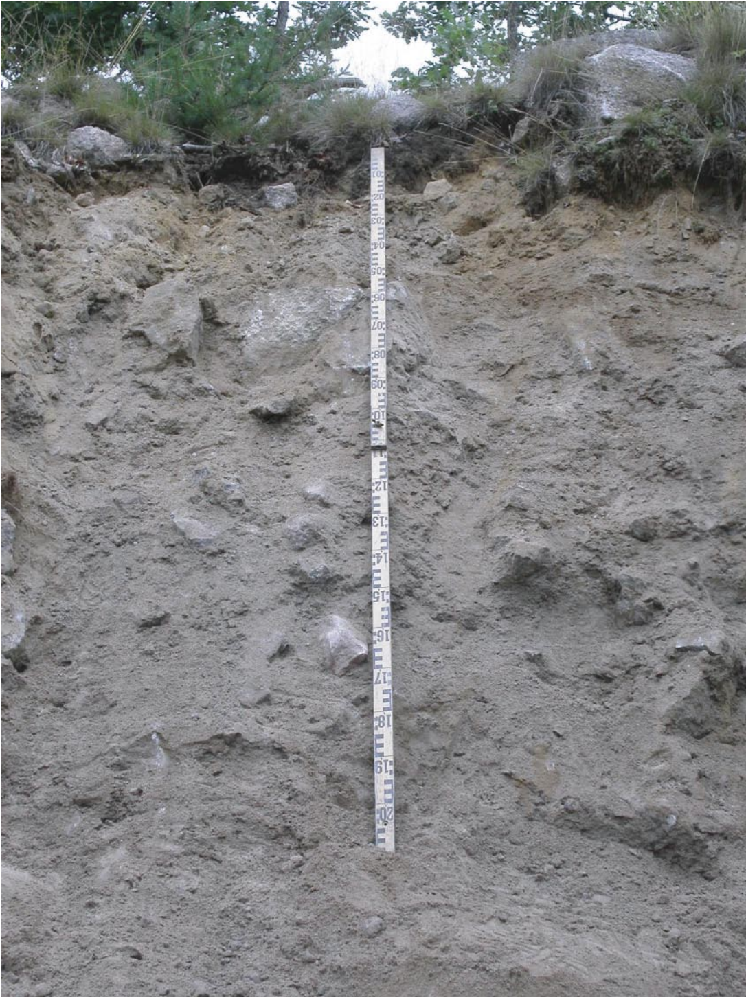
Figure 5-10. The upper part of a quarry section (PSM005413) displays 0.5 m of poorly consolidated flow till, underlain by at least 4 m of hard sandy basal till.
