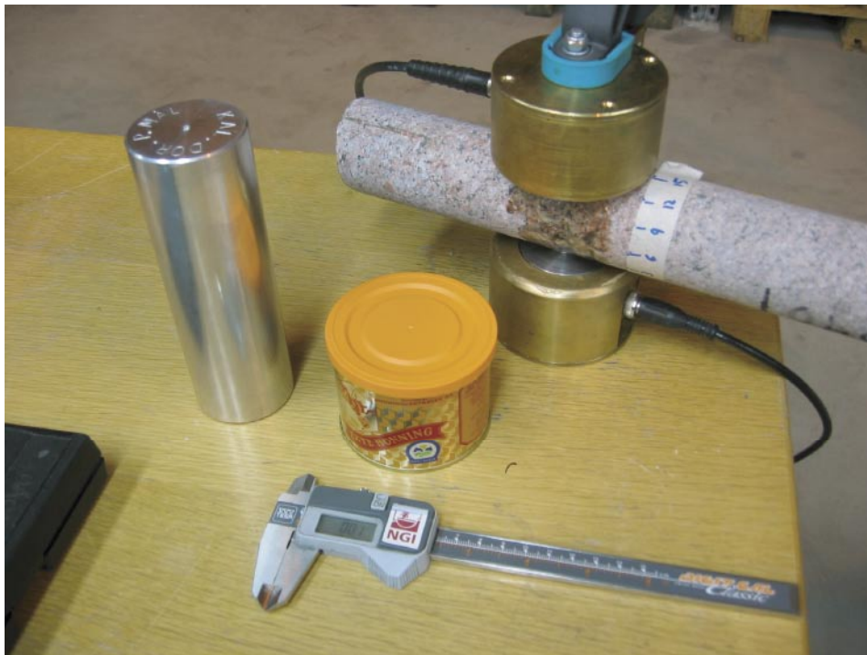
Figure 3-1. Detail of NGI's apparatus for measuring acoustic P-wave travel time transverse borehole core. The aluminium cylinder for calibration of the device is on the left.
