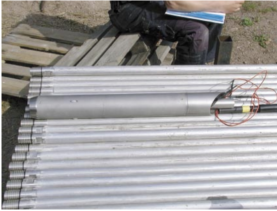
Photo 5: Positioner, bottom end of down-in-hole string
