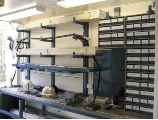
Photo 2: Rack for pump, down-hole equipment, workbench and drawers for tools.
