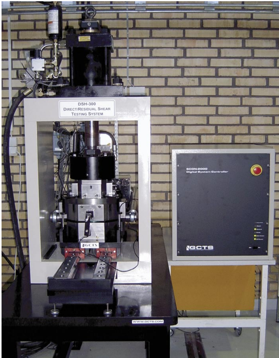
Figure 3-1. Equipment for direct shear tests and digital controller unit.
