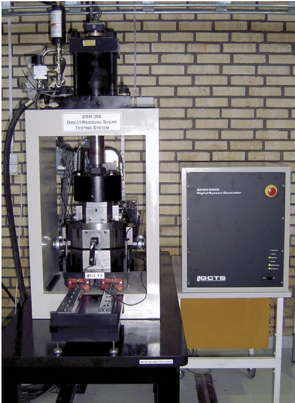
Figure 3-1. Equipment for direct shear tests: Load frame and digital controller unit.
