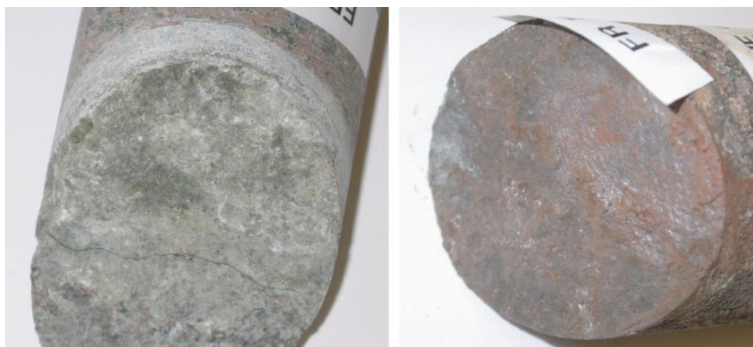
Figure 2-2. Fracture planes with chlorite+calcite and prehnite (left), and chlorite+calcite and hematite (right).
