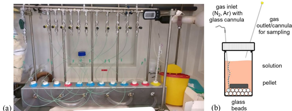
Fig. 1 a Experimental setup of the dissolution experiments. b Schematic drawing of the vessels for the accelerated dissolution experiments
